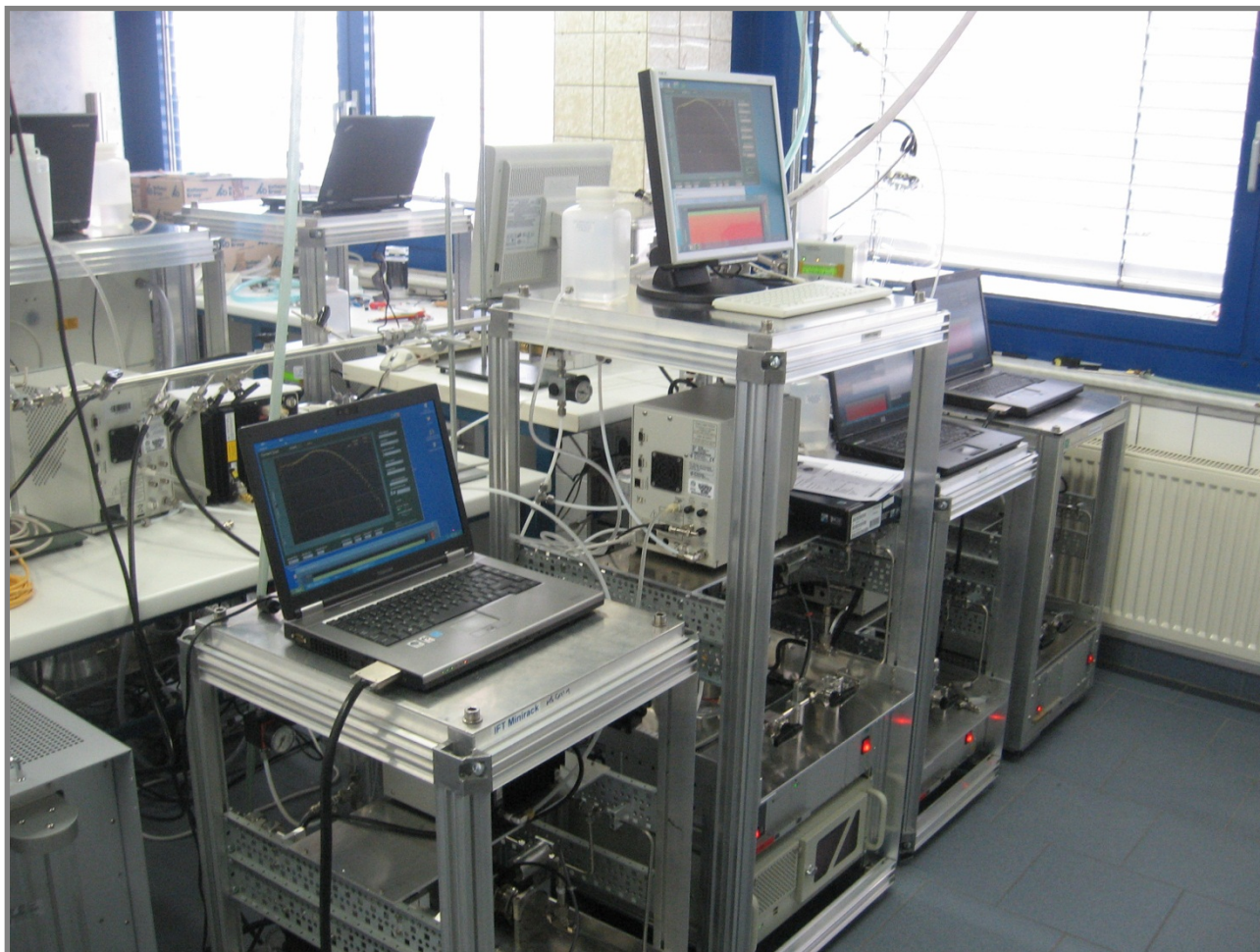
Figure 1: Comparison of different mobility particle size spectrometer at the IFT (Intercomparison workshop 2011)
